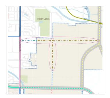
8. At the **Orchard & Pleasant Valley intersection**, shift the location of the roundabout off the sloped ground to level ground where a roundabout is less complicated and less costly to construct. Or add a note: "Actual roundabout location to be adjusted to due to topographic constraints".
